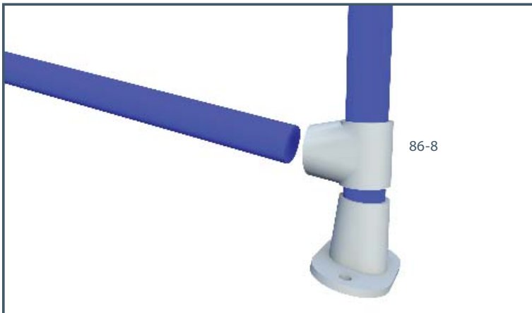
POST MOUNTED RAMP BOTTOM RAIL END: The bottom rail on a ramp terminates into a railing post using a 86-8. When the set screw is tightened, the angle of the bottom rail will be fixed.
