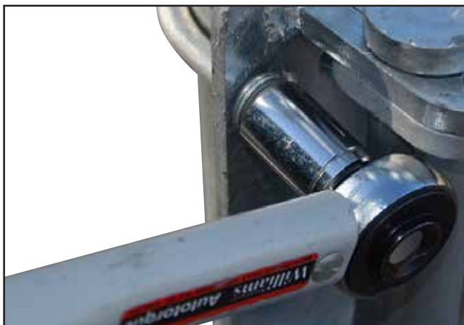
E. Torque all nuts/U-Bolts to 25Nm using the 13mm or 17mm socket and torque wrench.
